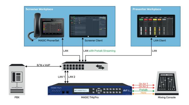
Our example application on this page shows a **basic setup of the MAGIC THipPro Telephone Hybrid**. There are two workplaces, one for the Presenter/Host and one for the Screener or Producer. The Screener/Producer works with the MAGIC THipPro Screener Software. He answers the calls first and can easily enter information about the callers via the data entry mask.
