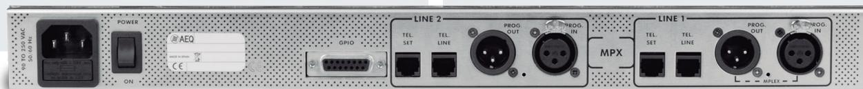
TH-03.2 AA: Two lines, analog inputs & outputs.
