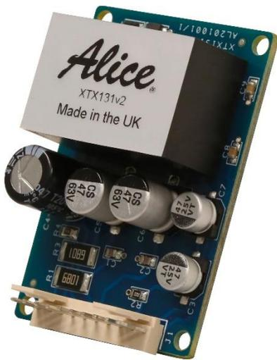
The Matchamp XTX131 v2 is a very high-performance balanced microphone amplifier module which achieves a noise performance which is typically less than 0.5dB from theoretical Johnson's noise when used with 150–200-ohm microphones.
