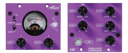
Set the 'output' at about 4. Set the meter switch to 'GR' (the meter needle will now sit at around the '0' point). Turn up the **COMPRESS** control slowly and, if there is enough audio signal, the meter will start to indicate compression by the needle moving downwards.
