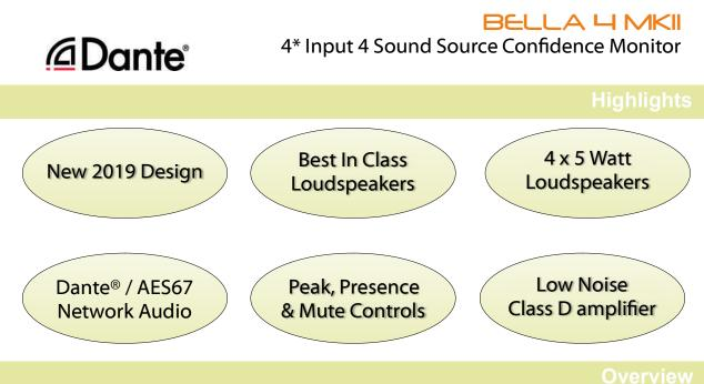
This device uses Audinate's Ultimo Chipset, which can receive 4 incoming audio channels, each at 48kHz. However, this chipset can only receive these 4 audio channels from a
