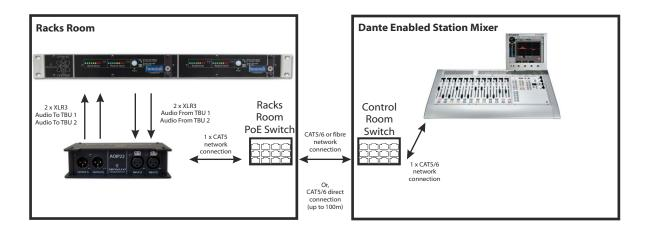
The AoIP22 is the perfect choice for installing in the back of a rack for interfacing legacy analogue audio equipment to your Dante network.
