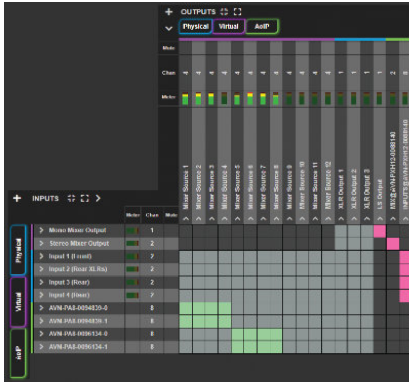
AVN-PXH12 GUI - The Audio Routing Grid on the 'Audio Routing' Web Page.
