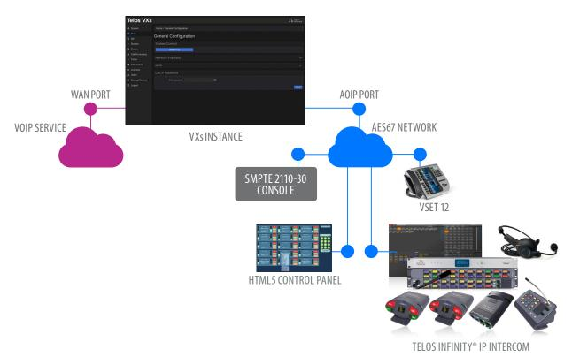
The diagram above shows an example system consisting of a Livewire+ audio console and Telos Infinity® IP Intercom.
